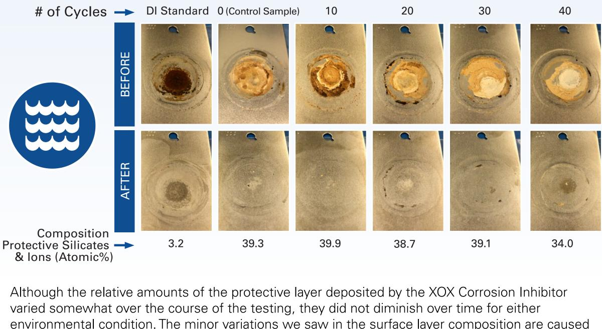
environmental condition. The minor variations we saw in the surface layer composition are caused by variations in the base chemistry of the insulation, and not by the material gaining or losing its corrosion inhibiting properties as a result of wet-dry cycling.
