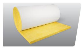
Micro-Flex® is a fiberglass wrap insulation for large diameter pipes and tanks. It is an alternative to pre-formed insulation. The fiber orientation of Micro-Flex enhances both the compressive strength and thermal performance when compared to conventional pipe and tank insulation. Micro-Flex rolls can be cut to size on-the-job and are available with an FSK or AP vapor-retarder facing. It provides a single solution to a variety of indoor and outdoor applications.
